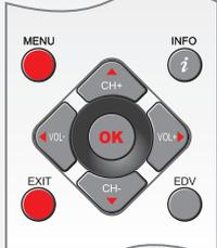
Press the MENU button to call up the main menu. Use the arrow buttons to navigate between the menu items and the OK button for selecting. Press the EXIT button to exit the menu structure.
