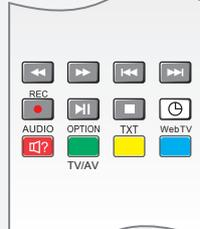
Depending on which column of the menu of the channel list you are, you can call up other functions and menus with the coloured buttons. These possible functions are displayed in the lower section.
