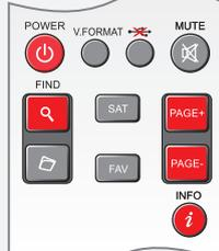
Use the Page button in the right column of the menu to scroll page by page through the channel lists. The INFO button displays information about a channel. The FIND button searches for channels.
