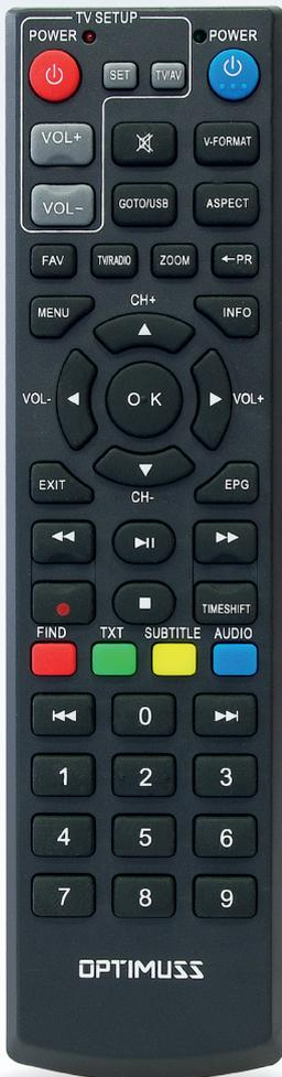
Your set-top-box remote control, with 5 learning-function keys and 1 “SET” key in the “TV panel” , is capable of learning the functions from your original TV remote control. Each of the 5 learning keys can learn any key of your original TV remote control. We recommend you to program the keys as Power, TV / AV, VOL+, VOL -, OK. The other 42 keys are for the control of the set-top-box.
