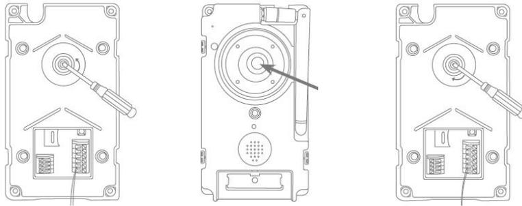
The door station's lens can be adjusted on the back by up to 7.5% vertically and 2.5% horizontally. To adjust the lens, loosen the screw using the triangle screwdriver provided. We recommend you first connect your intercom to the App2Cam Plus on your network before final installation in order to ensure it is perfectly positioned. Fix the position of the lens by tightening the screw on the rear of the bracket using the triangle screwdriver.
