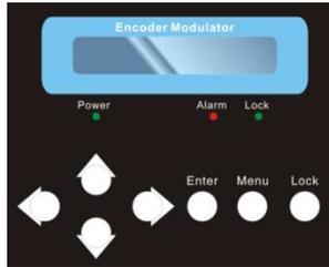
**LCD Display** – It presents the selected menu and the parameter settings. The backlight in the display is on when the power is applied.
