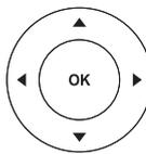
With the arrow keys you can scroll in the lists up and down, left and right or regulate the volume. With the OK-key you confirm your menu-entry or activate the channel-list.
