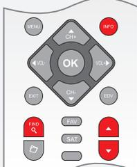
Use the Page button in the right column of the menu to scroll page by page through the channel lists. The INFO button displays information about a channel. The FIND button searches for channels.
