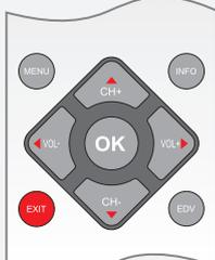
Press the OK button in TV or Radio mode to call up the channel list. Use the arrow buttons and OK button to navigate the menu. The EXIT button closes the list.
