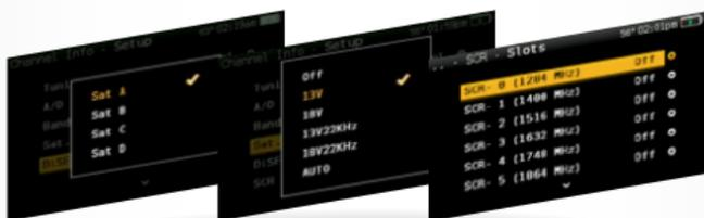
H30FLEX allows you to configure the parameters required for the reception of your satellite signal. To do this, H30FLEX allows pre-amplifier powering, **and configuration of both DiSeqC and SCR parameters.**
