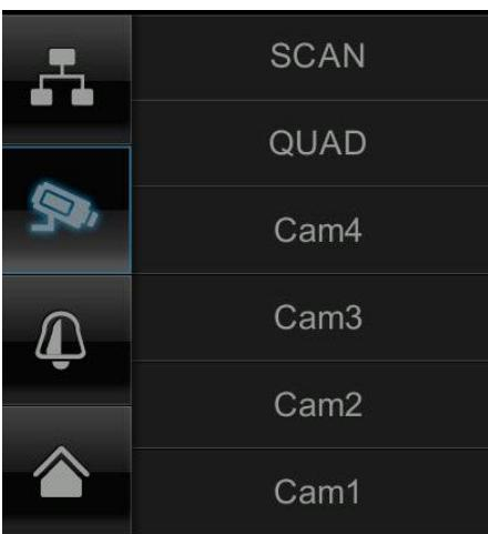
Select the required display mode, by pressing SCAN, QUAD or a camera (Cam1-4).
