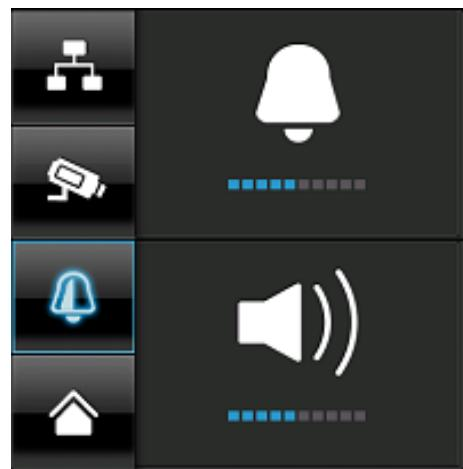
Set the volume of the alarm tone (bell symbol) or camera tone (loudspeaker symbol) by pressing “+” and “-”.
