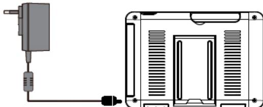
1. Connect the power supply unit to the monitor.
