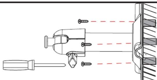
You can also swivel the mount by 90° into a particular position. First loosen the screw on the side and set the required angle. Then tighten the screw to secure the required position.
