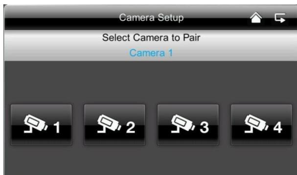
1. Select the required camera (1-4). The system counts down from 60 seconds.
