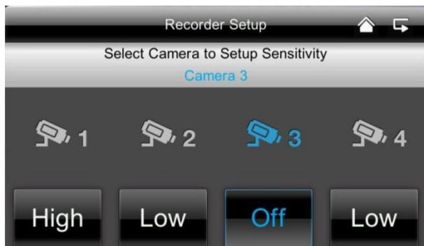
Here you can set the sensitivity of the motion detection for each camera.
