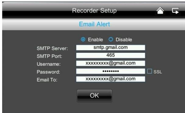
**!** To enable this function, the monitor must be in the docking station and connected to the internet.
