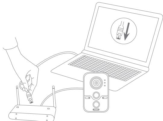
**Connecting the network camera to a router/switch**
