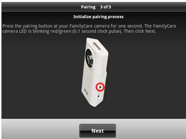
Follow the instructions on the screen and press and hold the pairing button on the camera. The Status LED on the camera starts flashing red and green. Now press "Next".
