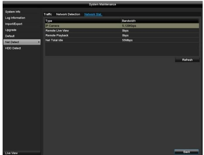
The bandwidth used by the device is displayed under this tab.
