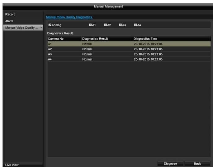
By pressing the "Diagnose" button, manual analysis is started. Adjust the settings under the Camera menu if the diagnose result produces an error message (blurred image, colour cast etc.) even if the image settings are correct.
