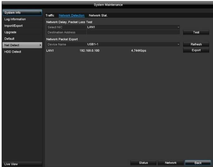
Under "Network Delay, Packet Loss Test", you can check the connection to another device, such as a computer ('pinging'). Enter the network address of the device to be checked (e.g. 192.168.0.25) and click on **Test**.
