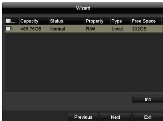
1. To set up a hard disk drive, enable the 'checkbox' with a left click and then click on **Init**.
