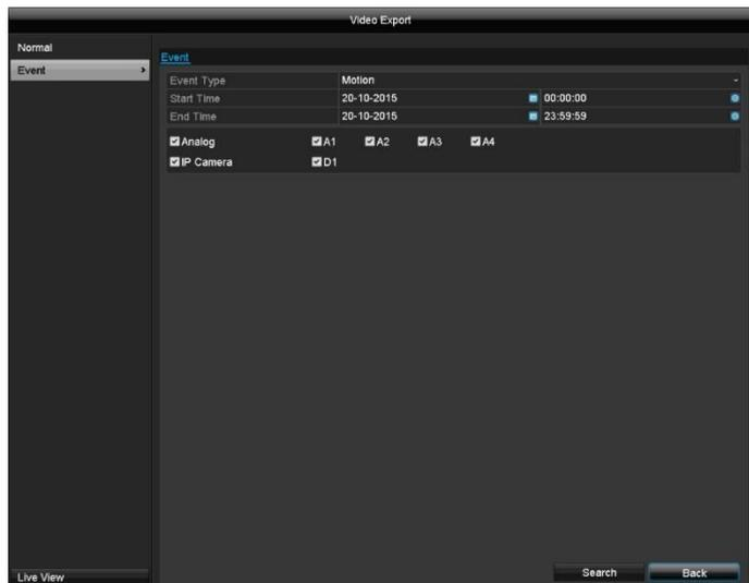
Define the period of the recordings to be searched for using the "Start Time" and "End Time" selection fields. Select the camera by ticking or unticking the box and then click on **Search**.
