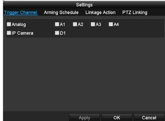
Tick the corresponding box to select which camera channel is triggered in the event of an alarm.
