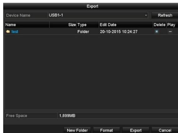
1. Select the connected medium to be used for storage from the drop-down menu.
