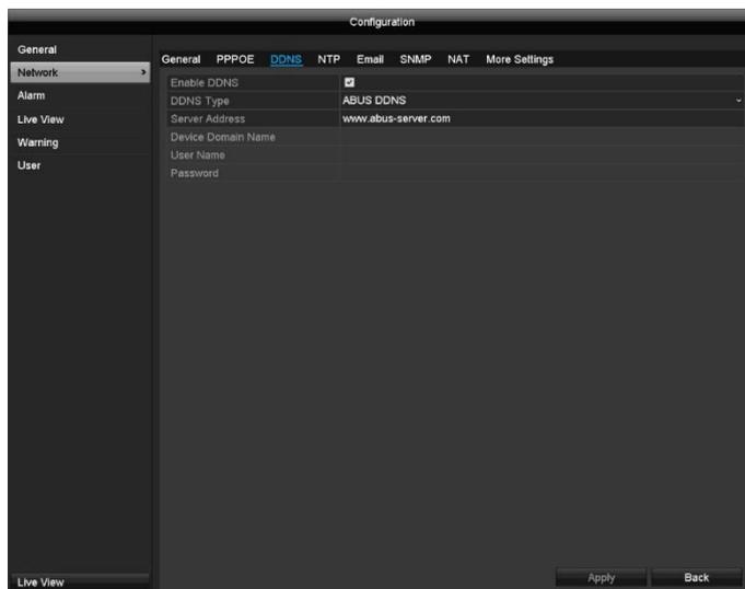
1. To be able to use the ABUS DDNS function, you first need to set up an account at [www.abus-server.com](http://www.abus-server.com). Please read the FAQs on this topic on the website.
