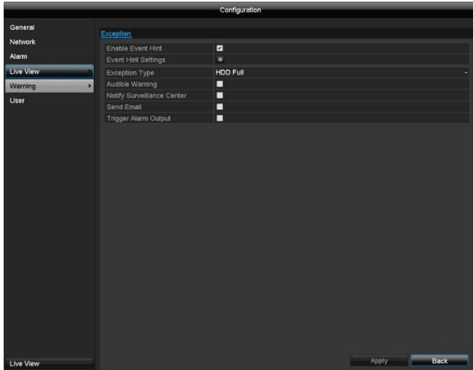
Set the response of the recorder for warning messages and system events here. To do this, activate the "Enable Event Hint" setting.
