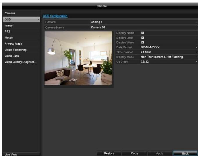
Select the camera channel to be processed under "Camera".
