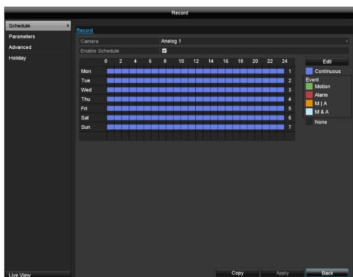
On the on-screen display, the hours for each day are listed from left to right, and the days are listed from top to bottom. On the right of the display, the colour key can be seen so, in the time schedule set up, the recording periods are displayed in the schedule in a different colour depending on the 'trigger' (recording type) in question.
