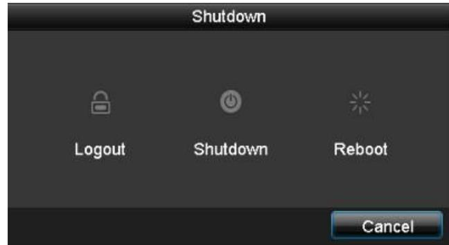
1. To switch off, select the **Shutdown** option and confirm the query with **Yes**. The device is switched off. Now pull out the plug of the power supply unit.
